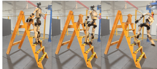
Figure 6: Failure case of the off-the-shelf teleoperation policy TWIST2 under ladder constraints.
