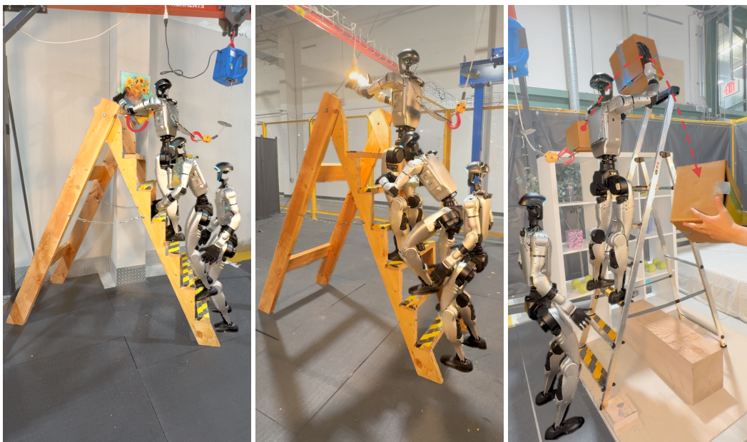
Figure 1: LadderMan enables a Unitree G1 humanoid to robustly climb diverse ladders using a single perceptive policy via zero-shot sim-to-real transfer. Building on the learned climbing capability, LadderMan further supports stable whole-body on-ladder manipulation via teleoperation, including adjusting paintings, replacing light bulbs, and box handover.
